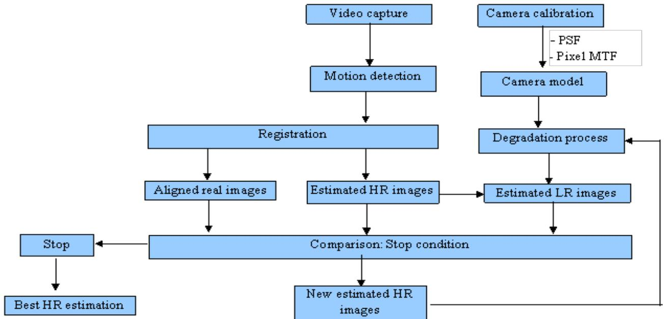
Figure 1: High-resolution processing block-diagram
