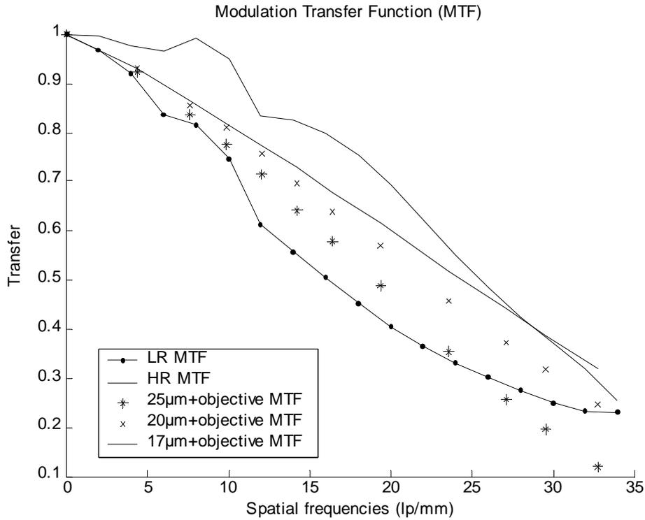
Figure 3: MTF for films with and without HR processing compared to various imaging system MTFs. We notice the good agreement between experimental data and theory in the 25µm case. The HR processing improves the system performance to make it nearly equivalent to a 15 to 17µm imaging system.
