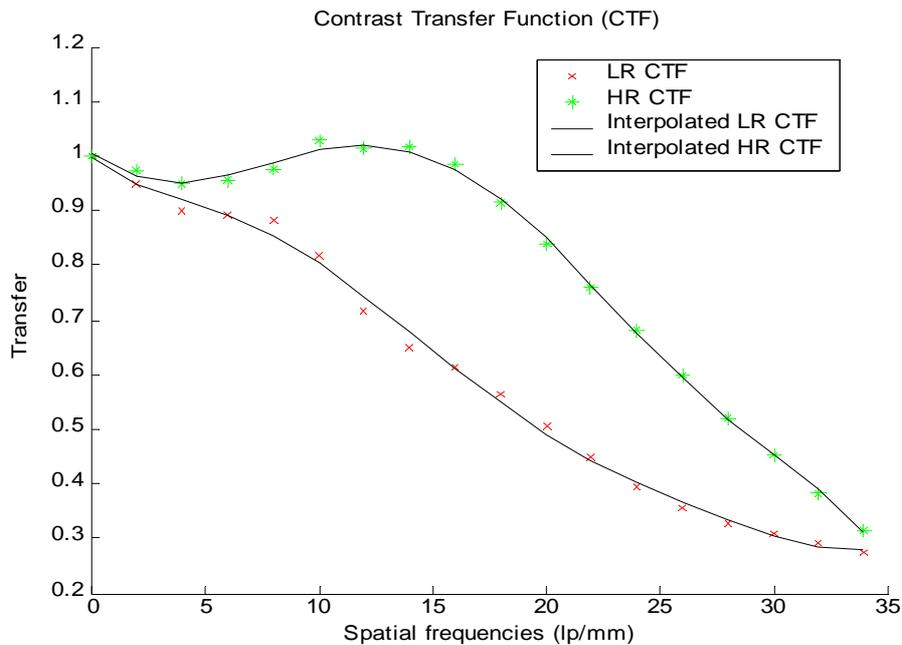
Figure 2: CTF computed with low resolution (LR) images and high resolution (HR) enhanced images.
